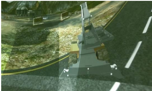
Fig 2. The projections are overlapping. In order to mask this effect, blending must be applied.
