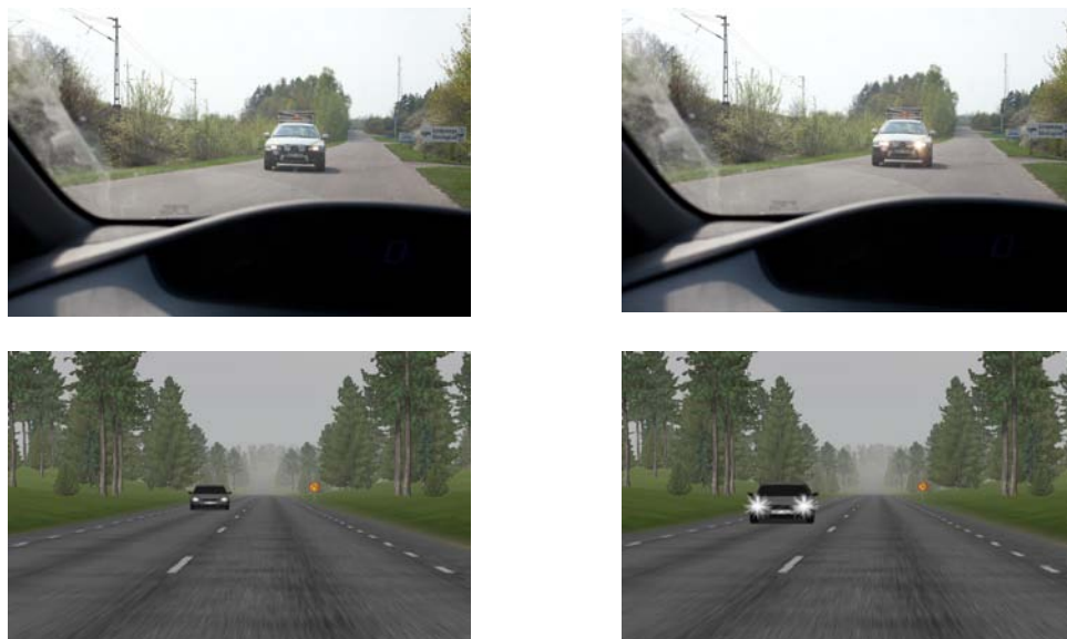
Figure 1: Photos of full and half beam are displayed for 20 meters distance along with an implementation in the simulator of a critical event with light warning thru a pulsed headlight from the POV.
