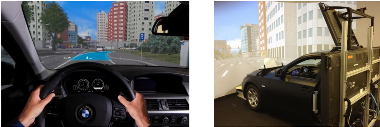
Fig. 6: Contact analogue lane marking and realization of head-up display in driving simulation
