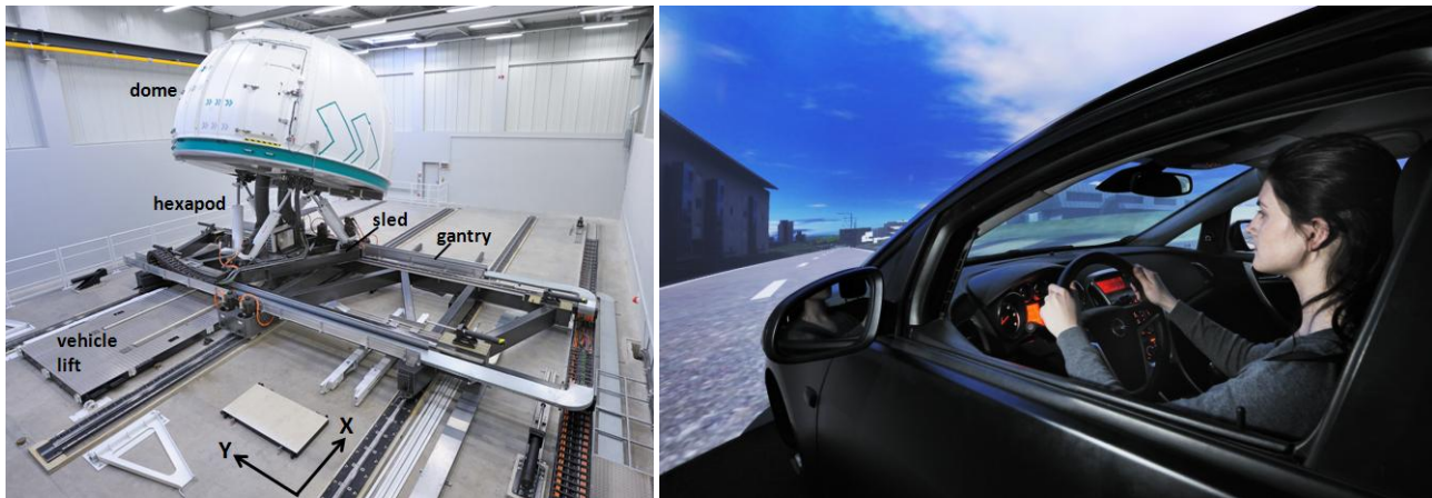
Fig. 1. Overall view and dome interior of the Stuttgart Driving Simulator
