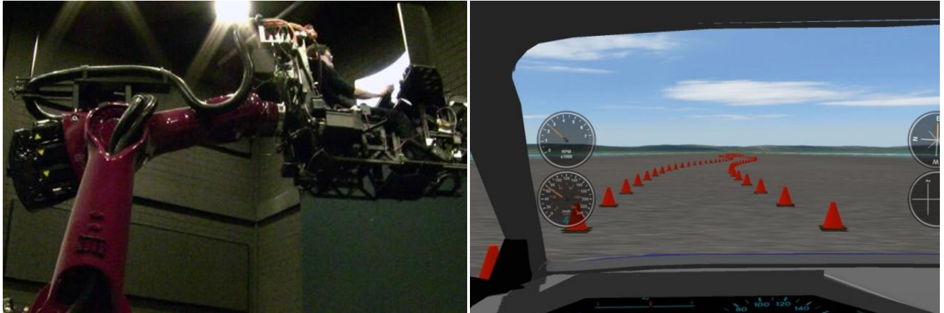
Fig. 1. MPI CyberMotion Simulator (a) and visual environment as seen from the driver (b).
