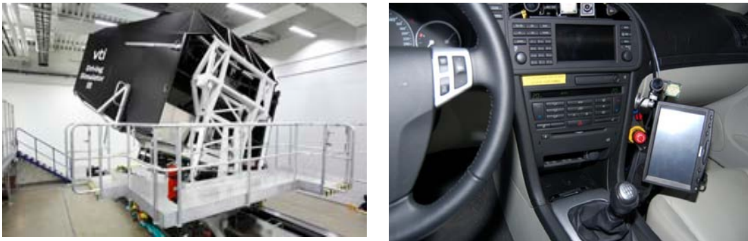
Figure 3: VTI's driving simulator III and the position of the visual distraction task display.
