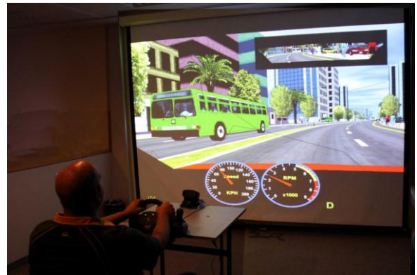
Fig. 1: The experiment setup. The participant seats in a clerical chair, holding the wheel. The scenario is presented on a wide screen in front of the participant.
